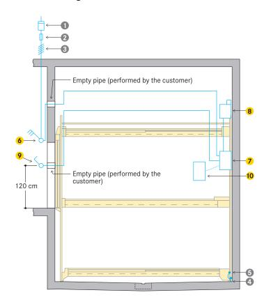
Cabling preparation to be performed by the customer:
