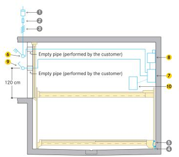
Cabling preparation to be performed by the customer:
