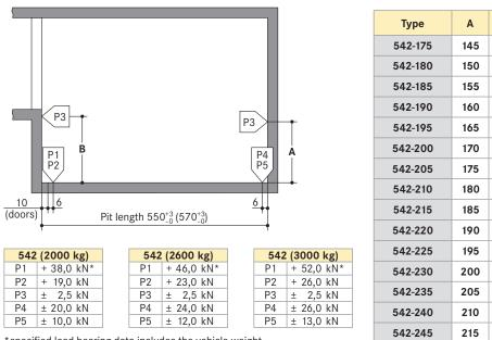
\*specified load bearing data includes the vehicle weight
